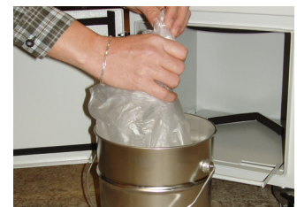
contamination free replacement of the filters by using the dust bag (included in delivery)
